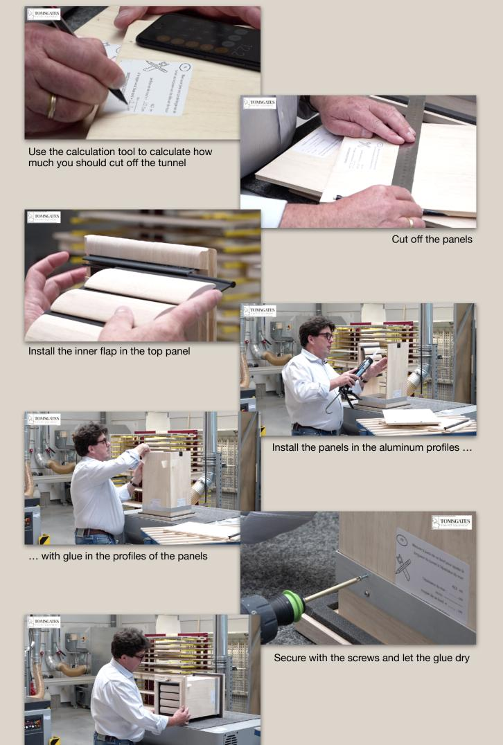
Install in the wall and finish with the frame
